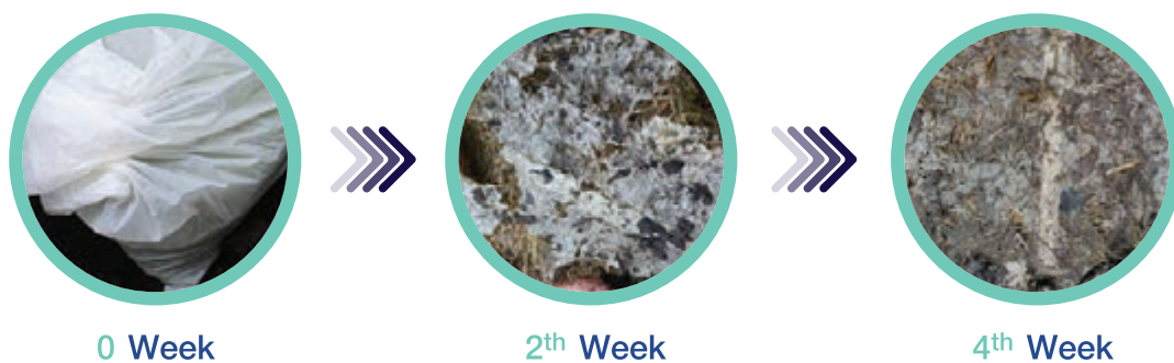
Testing the biodegradability of the bio-based components in ROSECO (according to ISO 16929 standard).
